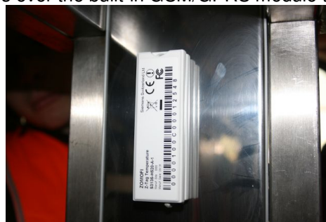
Fig 2: Transponder “Z-Tag Temperature” for long-range transmission
